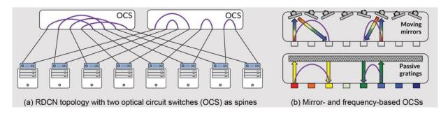
Concept of an optical circuit-switched spine layer. Here, top-of-rack switches connect to optical circuit switches (OCS) that dynamically create direct optical circuits between racks (purple arcs), rather than always sending traffic up through multiple electrical spine switches cacm.acm.org. In (b), examples of two OCS technologies are shown: one uses MEMS mirrors and another uses wavelength-based switching cacm.acm.org cacm.acm.org.
