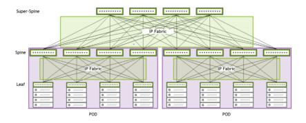
Example of a three-tier Clos network (leaf–spine–super-spine). Leaf/spine pods are aggregated via an additional super-spine layer to scale out the data center fabric docs.nvidia.com.
